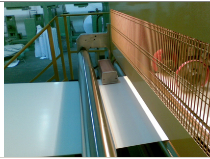
Model 1088 Sentinel® Splice Detector™ Pizzolato Sheeter
