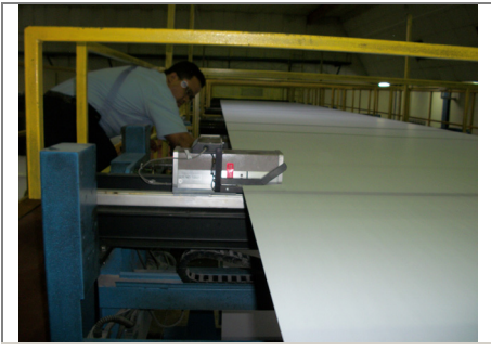
Model 1088 Sentinel® Splice Detector™ Jagenberg Sheeter
