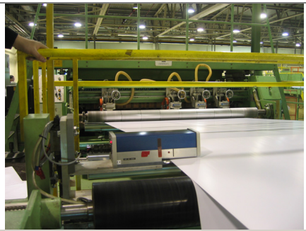
Model 1088 Sentinel® Splice Detector™ Jagenberg Sheeter
