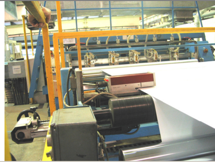
Model 1088 Sentinel® Splice Detector™ Strachen Henshaw Sheeter
