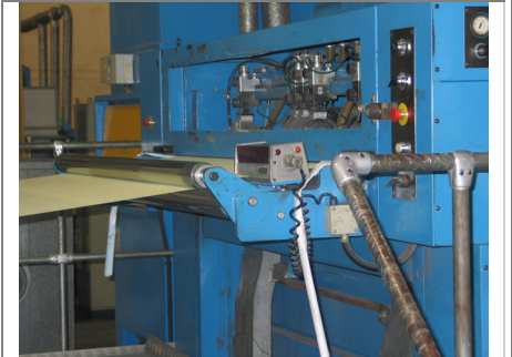
Model 1088 Sentinel® Splice Detector™ Strachen Henshaw Sheeter
